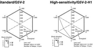
Conditions: Shock is applied in  $\pm X$ ,  $\pm Y$ , and  $\pm Z$  directions three times each with and without energizing the Relays to check the number of contact malfunctions.
