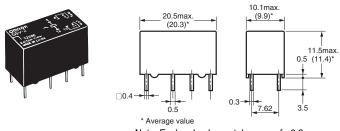
Note: Each value has a tolerance of ±0.3 mm.
