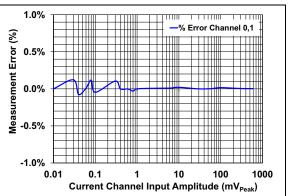
**FIGURE 2-6:** Measurement Error with 2-Point Calibration.
