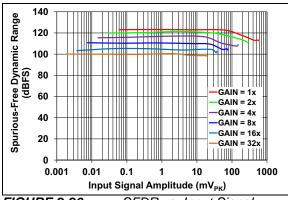
FIGURE 2-26: SFDR vs. Input Signal Amplitude.
