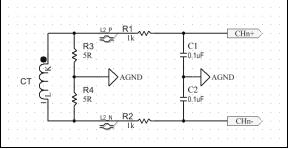
FIGURE 8-6: First-Order Anti-Aliasing Filter for CT-Based Designs.
