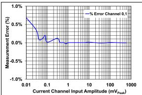
FIGURE 2-5: Measurement Error with 1-Point Calibration.
