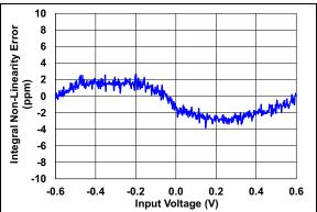
FIGURE 2-36: Integral Non-Linearity (Dithering Maximum).
