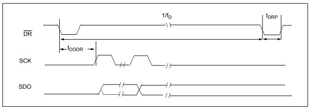
FIGURE 1-3: Data Ready Pulse/Sampling Timing Diagram.
