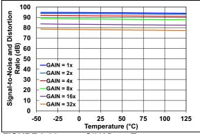
FIGURE 2-29: SINAD vs. Temperature.
