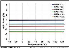
FIGURE 2-33: Gain Error vs. Temperature vs. Gain.
