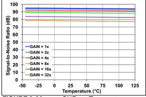
FIGURE 2-30: SNR vs. Temperature.
