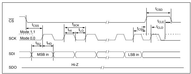
FIGURE 1-2: Serial Input Timing Diagram.
