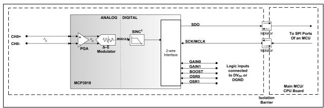
FIGURE 7-1: MCP3918 2-Wire Interface Typical Application Schematic.
