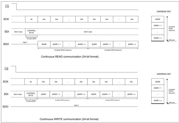
FIGURE 6-6: Continuous Communication Sequences.
