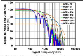
FIGURE 2-27: SINAD vs. Input Frequency.
