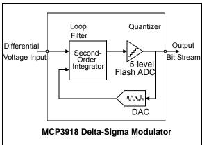
FIGURE 5-1: Simplified Delta-Sigma ADC Block Diagram.
