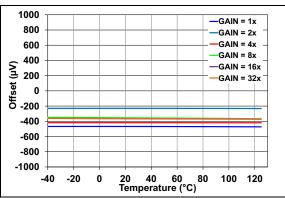
FIGURE 2-32: Offset vs. Temperature vs. Gain.
