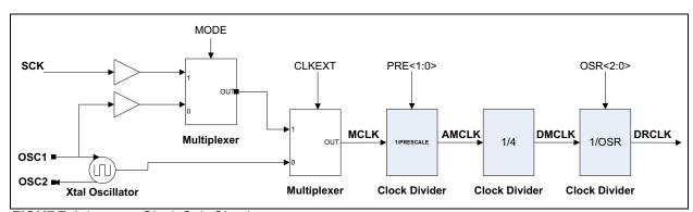
FIGURE 4-1: Clock Sub-Circuitry.
