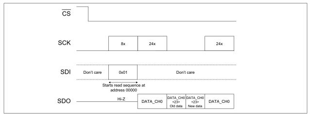
FIGURE 6-8: Typical Continuous Read Communication (WIDTH\_DATA<1:0> = 01, SPI Mode 1,1).
