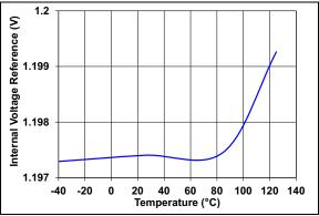
**FIGURE 2-34:** Internal Voltage Reference vs. Temperature.
