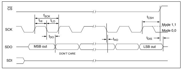
FIGURE 1-1: Serial Output Timing Diagram.
