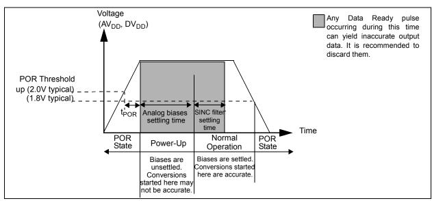
FIGURE 5-8: Power-On Reset Operation.
