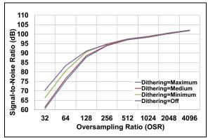
FIGURE 2-13: SNR vs.OSR.
