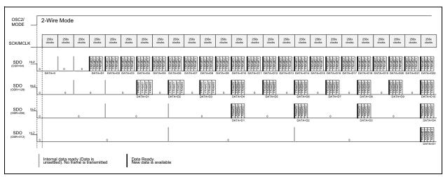
FIGURE 7-3: MCP3918 2-Wire Communication Protocol.
