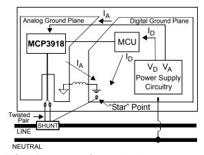
FIGURE 8-5: Connection Diagram.
