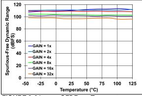
FIGURE 2-31: SFDR vs. Temperature.
