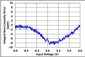
FIGURE 2-37: Integral Non-Linearity (Dithering Off).
