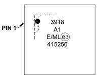
20-Lead SSOP (5.30 mm)
