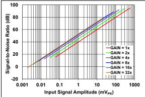
FIGURE 2-25: SNR vs. Input Signal Amplitude.
