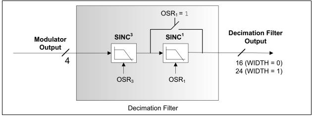
FIGURE 5-3: MCP3918 Decimation Filter Block Diagram.
