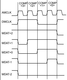
FIGURE 5-2: MDATO Serial Output with Respect to the Modulator Output Code.
