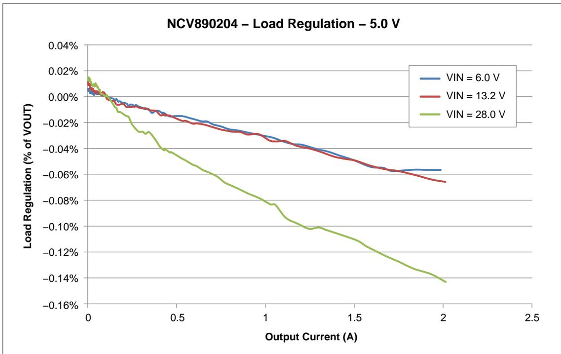
Figure 13. Load Regulation with a 5.0 V Output
