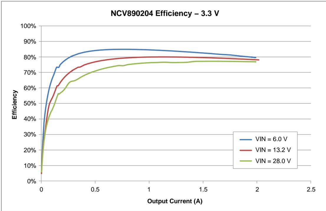
Figure 8. Efficiency with a 3.3 V Output
