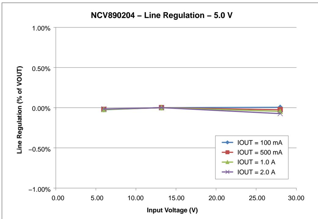
Figure 11. Line Regulation for a 5.0 V Output
