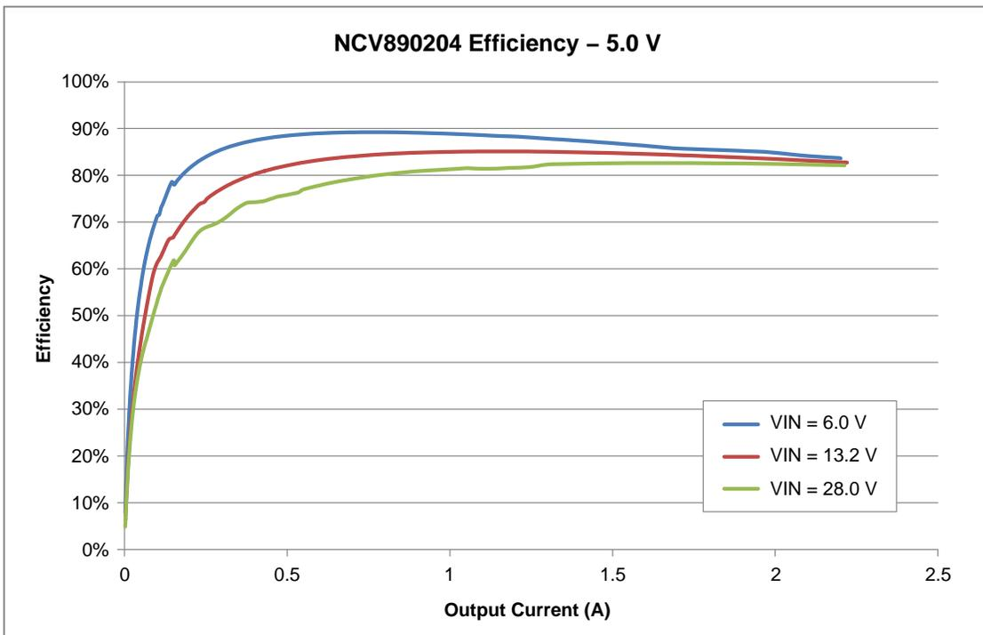
Figure 9. Efficiency with a 5.0 V Output
