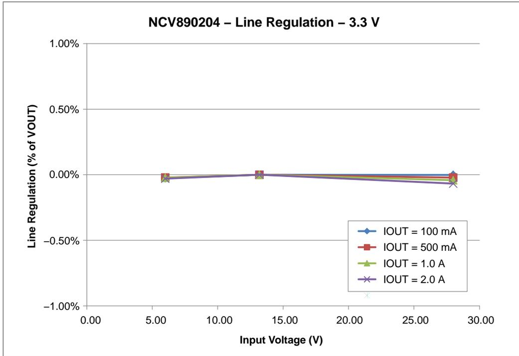
Figure 10. Line Regulation for a 3.3 V Output
