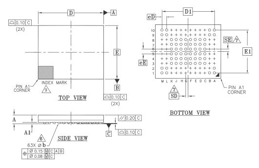
Figure 7.2 VBM063 — 63-Pin BGA, 11 mm x 9 mm Package
