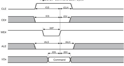
Figure 6.1 Command Latch Cycle
