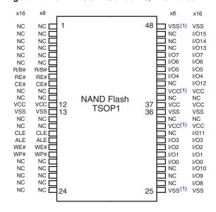
Figure 1.2 48-Pin TSOP1 Contact x8, x16 Device
