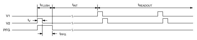
Figure 21. Pulse Flush Gate Timing
