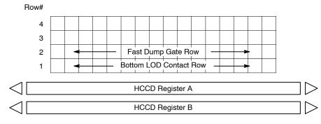
Figure 22. Fast Line Dump Layout
