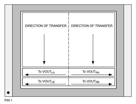
Figure 5. Image Transfer Diagram
