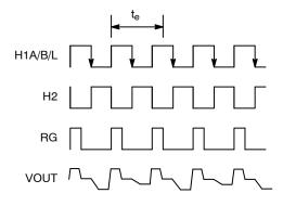
Figure 19. Pixel Timing
