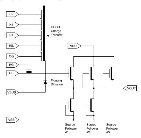
Figure 3. Output Architecture (Each Output)
