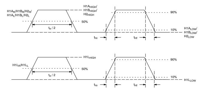
Figure 20. Pixel Timing Detail
