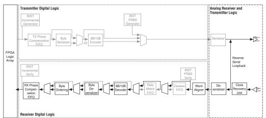
Figure 2–26 shows the data path in reverse serial loopback mode.
