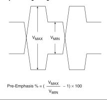
Pre-emphasis percentage is defined as  $(V_{MAX}/V_{MIN}-1) \times 100$ , where  $V_{MAX}$  is the differential emphasized voltage (peak-to-peak) and  $V_{MIN}$  is the differential steady-state voltage (peak-to-peak).
