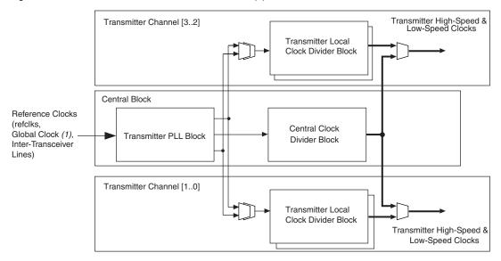
Figure 2–3. Clock Distribution for the Transmitters Note (1)
