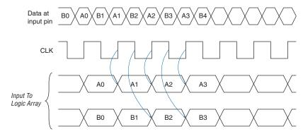
When using the IOE for DDR outputs, the two output registers are configured to clock two data paths from ALMs on rising clock edges. These output registers are multiplexed by the clock to drive the output pin at a  $\times 2$  rate. One output register clocks the first bit out on the clock high time, while the other output register clocks the second bit out on the clock low time. Figure 2–84 shows the IOE configured for DDR output. Figure 2–85 shows the DDR output timing diagram.
