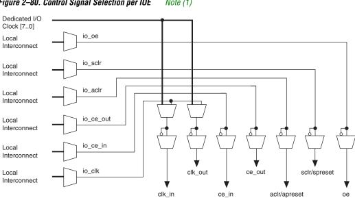
Figure 2-80. Control Signal Selection per IOE Note (1)
