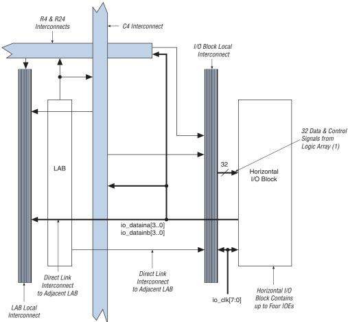
Figure 2-77. Row I/O Block Connection to the Interconnect
