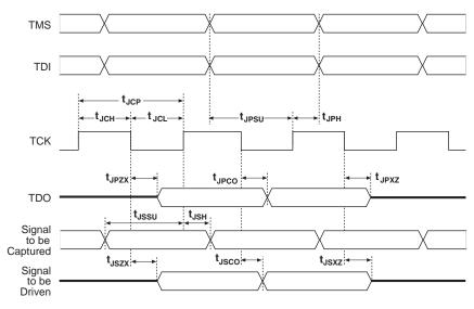
Table 4–117 shows the JTAG timing parameters and values for Stratix II GX devices.
