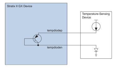
Figure 3-1. External Temperature-Sensing Diode
