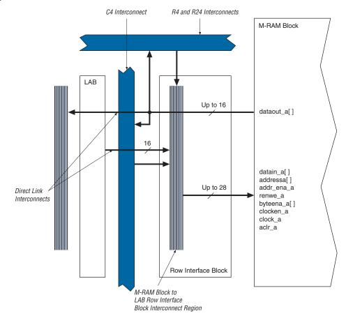
Figure 2-56. M-RAM Row Unit Interface to Interconnect
