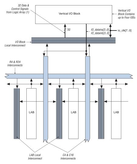
Figure 2–78 shows how a column I/O block connects to the logic array.
