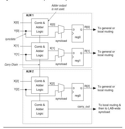
Figure 2-42. Conditional Operation Example
