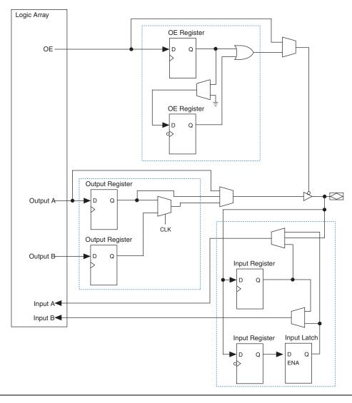
Figure 2-76. Stratix II GX IOE Structure
