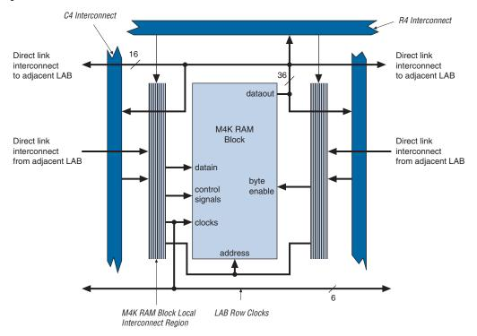
Figure 2-52. M4K RAM Block LAB Row Interface
