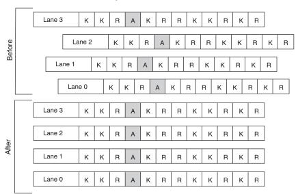
Figure 2-19. Before and After the Channel Aligner
