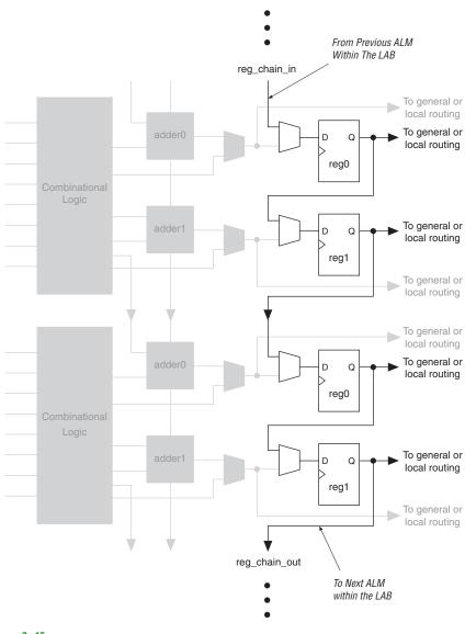
Figure 2–45. Register Chain within a LAB Note (1)
