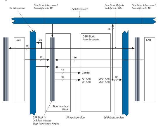
Figure 2-60. DSP Block Interface to Interconnect
