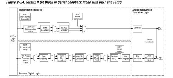
Figure 2–24 shows the data path in serial loopback mode.
