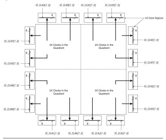
Figure 2-66. EP2SGX60, EP2SGX90 and EP2SGX130 Device I/O Clock Groups
