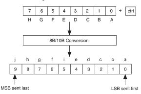
In single-width mode, the 8B/10B encoder generates a 10-bit code group from the 8-bit data and 1-bit control identifier. In double-width mode, there are two 8B/10B encoders that are cascaded together and generate a 20-bit (2 × 10-bit) code group from the 16-bit (2 × 8-bit) data + 2-bit (2 × 1-bit) control identifier. Figure 2–6 shows the 20-bit encoding process. The 8B/10B encoder conforms to the IEEE 802.3 1998 edition standards.
