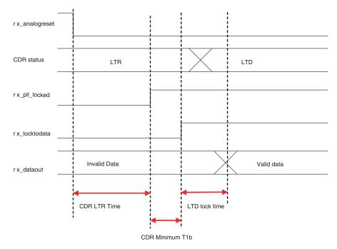
Figure 4-2. Lock Time Parameters for Automatic Mode
