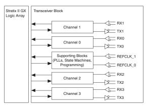
Figure 2-2. Elements of the Transceiver Block
