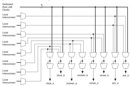
Figure 2-51. M4K RAM Block Control Signals
