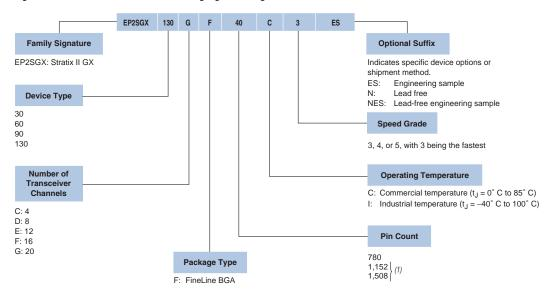
Figure 5-1. Stratix II GX Device Packaging Ordering Information
