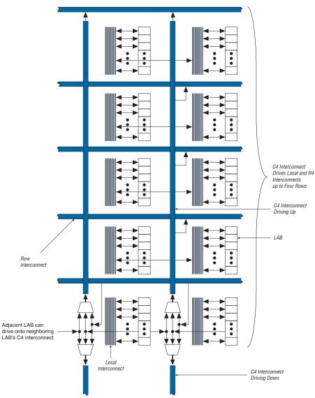
Figure 2–48. C4 Interconnect Connections Note (1)
