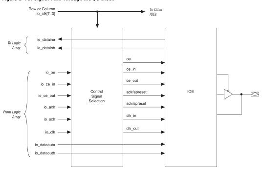
Figure 2-79. Signal Path Through the I/O Block
