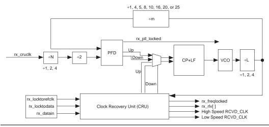
The receiver PLLs and CRUs can support frequencies up to 6.375 Gbps. The input clock frequency is limited to the full clock range of 50 to 622 MHz but only when using REFCLKO or REFCLK1. An optional RX\_PLL\_LOCKED port is available to indicate whether the PLL is locked to the reference clock. The receiver PLL has a programmable loop bandwidth which can be set to low, medium, or high. The Quartus II software can statically set the loop bandwidth parameter.
