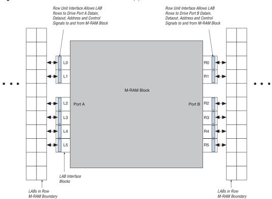
Figure 2–55. M-RAM Block LAB Row Interface Note (1)
