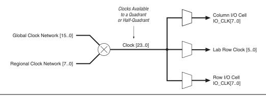
IOE clocks have row and column block regions that are clocked by  $8\,\mathrm{I/O}$  clock signals chosen from the 24 quadrant clock resources. Figures 2–65 and 2–66 show the quadrant relationship to the I/O clock regions.
