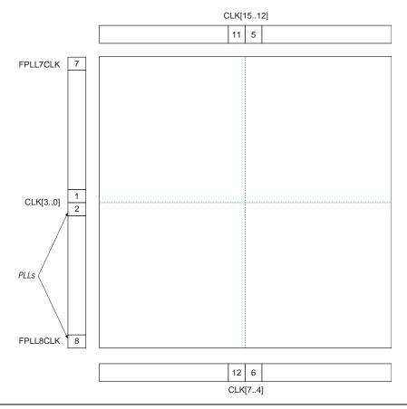
Figures 2–71 and 2–72 shows global and regional clocking from the fast PLL outputs and the side clock pins. The connections to the global and regional clocks from the fast PLL outputs, internal drivers, and the CLK pins on the left side of the device are shown in Table 2–27.
