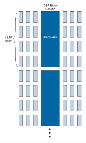
Table 2–21 shows the number of DSP blocks in each Stratix II GX device. DSP block multipliers can optionally feed an adder/subtractor or accumulator in the block, depending on the configuration, which makes routing to ALMs easier, saves ALM routing resources, and increases performance because all connections and blocks are in the DSP block.
