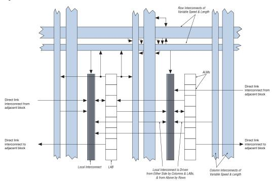
Figure 2-32. Stratix II GX LAB Structure
