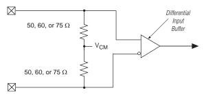
If a design uses external termination, the receiver must be externally terminated and biased to 0.85 V or 1.2 V. Figure 2–14 shows an example of an external termination and biasing circuit.
