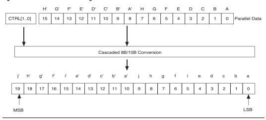
Upon power on or reset, the 8B/10B encoder has a negative disparity which chooses the 10-bit code from the RD-column. However, the running disparity can be changed via the tx\_forcedisp and tx\_dispval ports.
