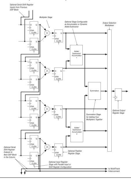
Figure 2-58. DSP Block Diagram for 18 x 18-Bit Configuration
