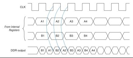
The Stratix II GX IOE operates in bidirectional DDR mode by combining the DDR input and DDR output configurations. The negative-edge-clocked OE register holds the OE signal inactive until the falling edge of the clock to meet DDR SDRAM timing requirements.
