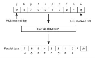
The 8B/10B decoder in double-width mode translates the 20-bit (2  $\times$  10-bits) encoded code into the 16-bit (2  $\times$  8-bits) equivalent data or control code. The 20-bit upper and lower symbols received must be from the supported Dx.y or Kx.y list with the proper disparity or error flags
