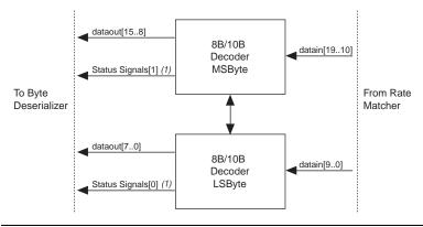
The 8B/10B decoder in single-width mode translates the 10-bit encoded data into the 8-bit equivalent data or control code. The 10-bit code received must be from the supported Dx.y or Kx.y list with the proper disparity or error flags asserted. All 8B/10B control signals, such as disparity error or control detect, are pipelined with the data and edge-aligned with the data. Figure 2–22 shows how the 10-bit symbol is decoded in the 8-bit data + 1-bit control indicator.
