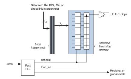
Figure 2-88. Stratix II GX Transmitter Channel
