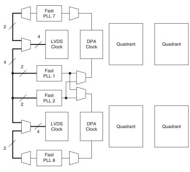
Figure 2–91. Fast PLL and Channel Layout in the EP2SGX60E to EP2SGX130 Devices Note (1)
