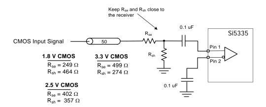
Figure 10. Interfacing CMOS Reference Clocks to the Si5335
