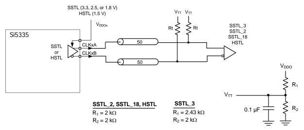
Figure 16. Interfacing the Si5335 to an SSTL or HSTL Receiver
