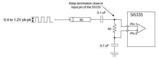
Figure 12. Single-Ended Input Signal with 50  $\Omega$  Termination
