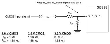
Figure 13. P5, P6 Control Pin Termination
