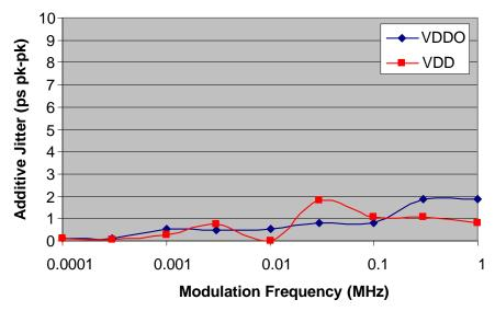
Figure 24. Peak-to-Peak Additive Jitter from 100 mV Sine Wave on Supply
