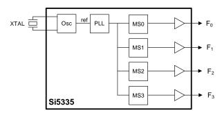
Figure 25. Si5335 as a Free-Running Clock Generator
