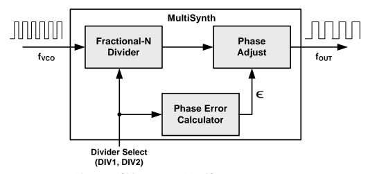
Figure 3. Silicon Labs' MultiSynth Technology
