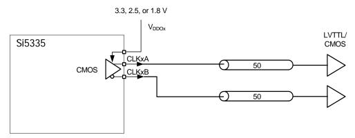
Figure 15. Interfacing to a CMOS Receiver
