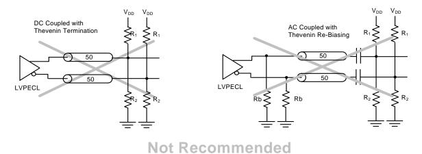
Figure 7. Common LVPECL Connections that May be Destructive to the Si5335 Input
