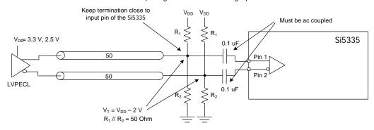
LVPECL Input Signal with Load Biasing Option
