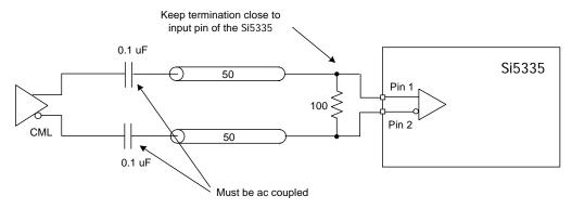
Figure 8. CML Input Signal
