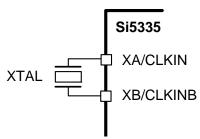
Figure 4. Connecting an XTAL to the Si5335
