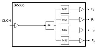
Figure 26. Si5335 as a Synchronous Clock Generator or Frequency Translator
