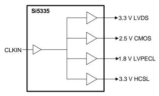
Figure 27. Si5335 as a Configurable Clock Buffer with Level Translation
