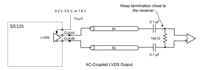
Figure 19. Interfacing to an LVDS Receiver
