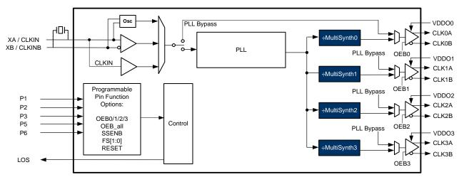
Figure 2. Si5335 Functional Block Diagram
