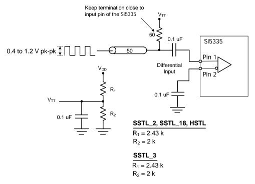
Figure 11. Single-Ended SSTL/HSTL Input Clocks to the Si5335
