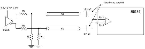
Figure 9. HCSL Input Signal to Si5335
