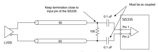
Figure 5. LVDS Input Signal
