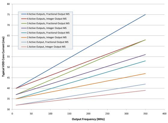
Figure 22. Core VDD Supply Average Current vs Output Frequency
