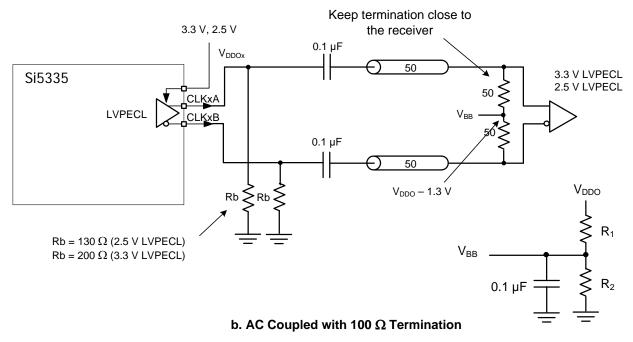
Figure 18. Interfacing to an LVPECL Receiver Using AC Coupling
