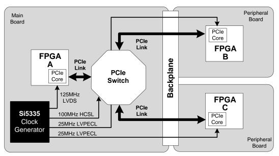
Figure 1. PCI Express Switching Application Example
