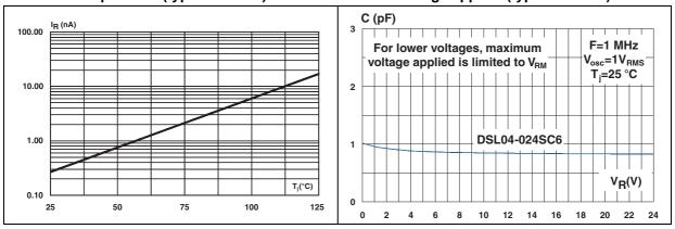
Figure 4. I / V characteristics (typical values)
