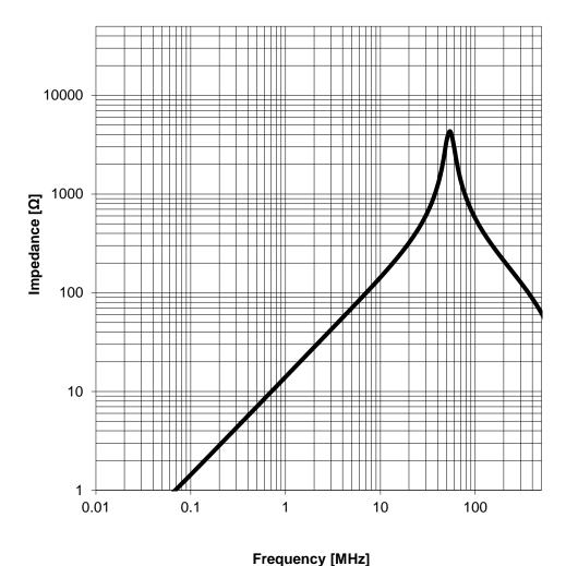
GENERAL TOLERANCE CREATED CHECKED Würth Elektronik eiSos GmbH & Co. KG EMC & Inductive Solutions SSt SSt DIN ISO 2768-1m Max-Eyth-Str. 1 74638 Waldenburg **WE-MAPI SMD Shielded Power** Tel. +49 (0) 79 42 945 - 0 Inductor ORDER CODE www.we-online.com 74438323022 eiSos@we-online.com REVISION STATUS BUSINESS UNIT PAGE Valid 3/7 001.002 2015-11-10 eiSos 2510 **WÜRTH ELEKTRONIK**
