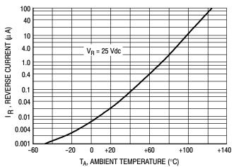
Figure 4. Leakage Current
