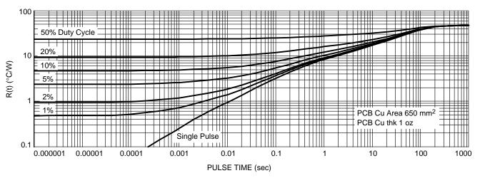
Figure 13. Thermal Characteristics
