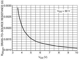
Figure 3. On-Resistance vs. V<sub>GS</sub>
