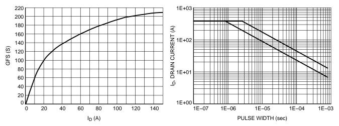
Figure 14. GFS vs. I<sub>D</sub>
