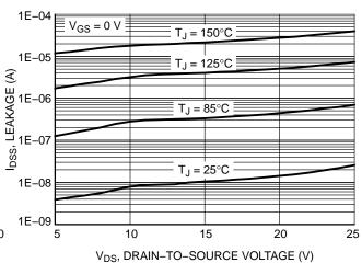
Figure 6. Drain-to-Source Leakage Current vs. Voltage
