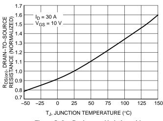
Figure 5. On–Resistance Variation with Temperature
