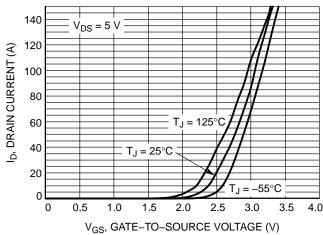
Figure 2. Transfer Characteristics
