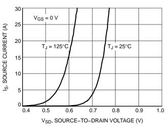
Figure 10. Diode Forward Voltage vs. Current
