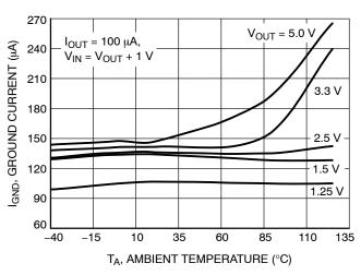
Figure 18. Ground Current vs. Temperature (V<sub>out</sub> = 1.25 V, 1.5 V, 2.5 V, 3.3 V, 5.0 V)
