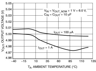
Figure 15. Output Voltage vs. Temperature (V<sub>out</sub> = 5.0 V)
