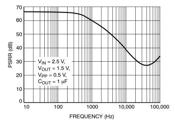
Figure 31. PSRR vs. Frequency (V<sub>out</sub> = 1.5 V)
