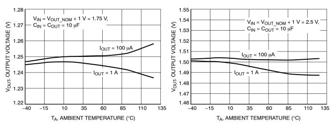
Figure 11. Output Voltage vs. Temperature (V<sub>out</sub> = 1.25 V)
