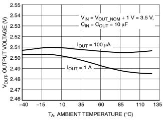
Figure 13. Output Voltage vs. Temperature  $(V_{out} = 2.5 \text{ V})$
