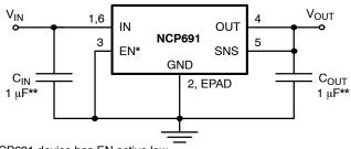
Note: \* NCP691 device has EN active low \*\* Minimum value required for stability
