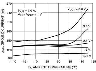
Figure 17. Ground Current vs. Temperature (V<sub>out</sub> = 1.25 V, 1.5 V, 2.5 V, 3.3 V, 5.0 V)
