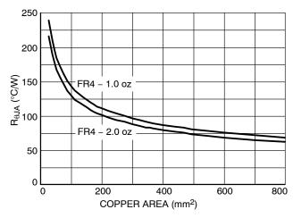
Figure 32. Thermal Resistance vs. Copper Area
