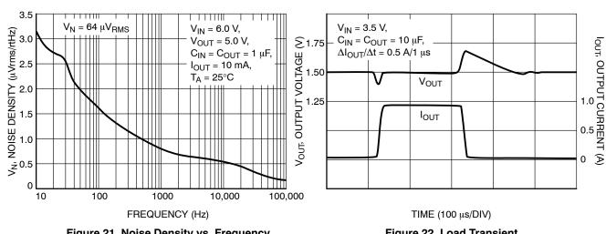
Figure 21. Noise Density vs. Frequency (V<sub>out</sub> = 5.0 V)
