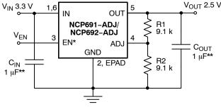
Note: \* NCP691-ADJ device has EN active low and NCP692-ADJ device has EN active high \*\* Minimum value required for stability
