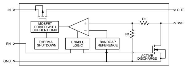
Figure 7. NCP692 Block Diagram (Fixed Version)
