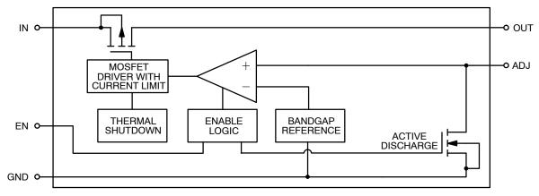
Figure 10. NCP692 Block Diagram (Adjustable Version)
