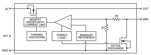
Figure 5. NCP690, NCV8690 Block Diagram (Fixed Version)
