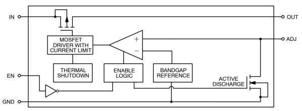
Figure 9. NCP691 Block Diagram (Adjustable Version)
