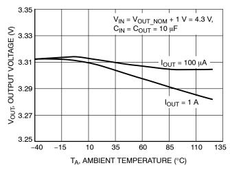
Figure 14. Output Voltage vs. Temperature  $(V_{out} = 3.3 \text{ V})$
