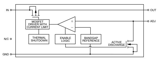
Figure 8. NCP690, NCV8690 Block Diagram (Adjustable Version)
