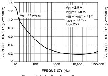
Figure 19. Noise Density vs. Frequency (V<sub>out</sub> = 1.5 V)
