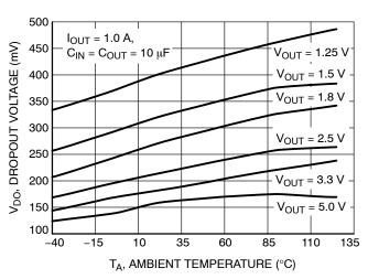
Figure 16. Dropout Voltage vs. Temperature (V<sub>out</sub> = 1.25 V, 1.5 V, 1.8 V, 2.5 V, 3.3 V, 5.0 V)
