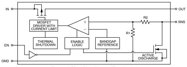
Figure 6. NCP691 Block Diagram (Fixed Version)
