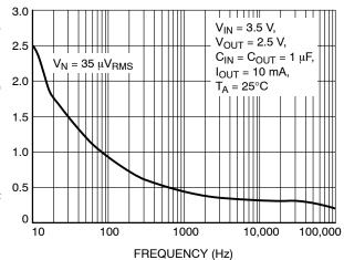
Figure 20. Noise Density vs. Frequency (V<sub>out</sub> = 2.5 V)
