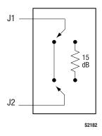
Figure 1. AA116-72LF Block Diagram
