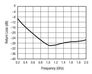
Figure 6. Return Loss in Attenuation State vs Frequency
