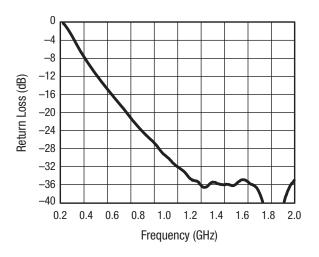
Figure 4. Return Loss in Insertion Loss State vs Frequency
