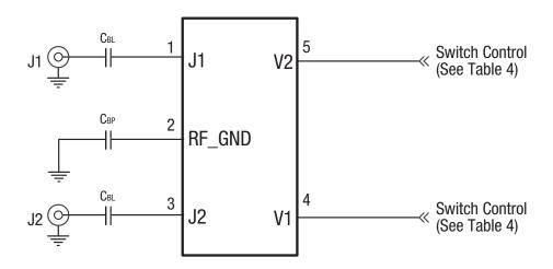
Note: CBL = 33 pF, CBP = 39 pF for 900 MHz operation. CBL = 100 nF, CBP = 100 nF for 0.004 to 0.05 GHz operation.
