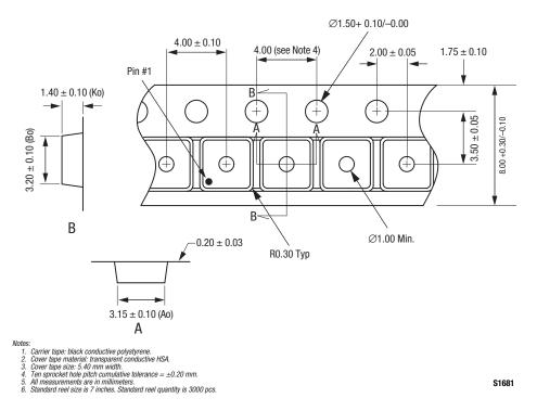
Figure 11. AA116-72LF Tape and Reel Dimensions
