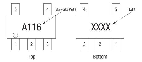
**Figure 9. Typical Part Markings**
