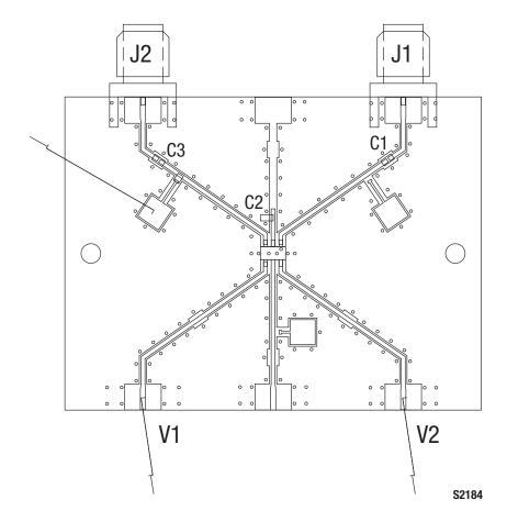
Figure 7. AA116-72LF Evaluation Board Assembly Diagram
