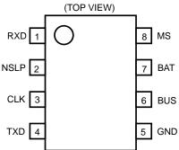
Figure 2. Pin Configuration
