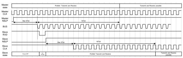
Figure 14. The Actual Time of Transmission and Reception after "CODEC Mode" Changing
