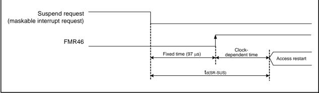
Figure 5.2 **Transition Time to Suspend**
