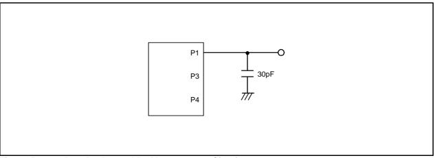
Figure 5.1 Port P1, P3, and P4 Measurement Circuit
