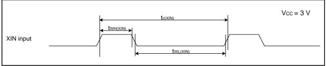
Figure 5.13 XIN Input Timing Diagram when VCC = 3 V
