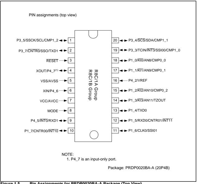
Figure 1.5 Pin Assignments for PRDP0020BA-A Package (Top View)
