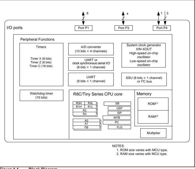
Figure 1.1 Block Diagram
