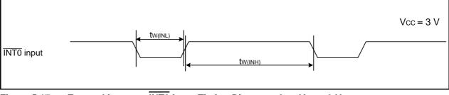
Figure 5.17 External Interrupt INTO Input Timing Diagram when Vcc = 3 V
