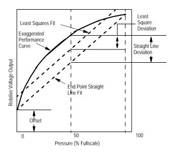
Figure 2. Linearity Specification Comparison
