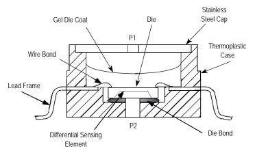
Figure 4. Cross-Sectional Diagram (Not to Scale)
