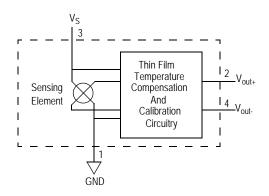
Figure 1. Temperature Compensated Pressure Sensor Schematic
