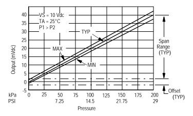
Figure 3. Output versus Pressure Differential
