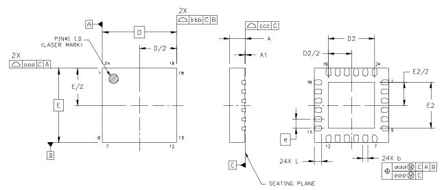
Figure 4. 24-Lead Quad Flat No-Lead (QFN)
