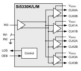
Figure 1. Si5330 Functional Block Diagrams
