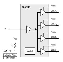
Figure 2. LOS Indicator with External Pull-Up
