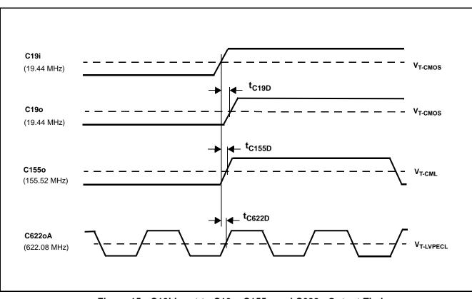
Figure 15 - C19i Input to C19o, C155o and C622o Output Timing
