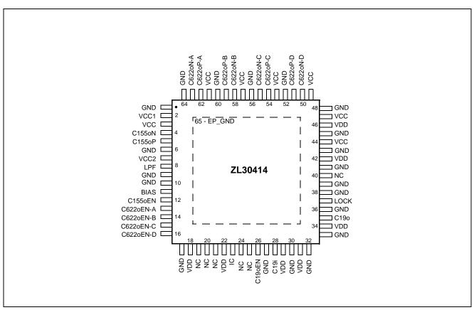
Figure 2 - TQFP 64 pin (Top View)
