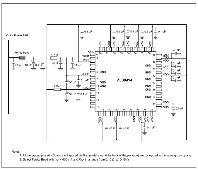
Figure 13 - Power Supply and BIAS Circuit Filtering
