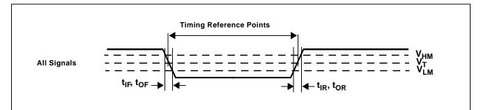
Figure 14 - Output Timing Parameter Measurement Voltage Levels
