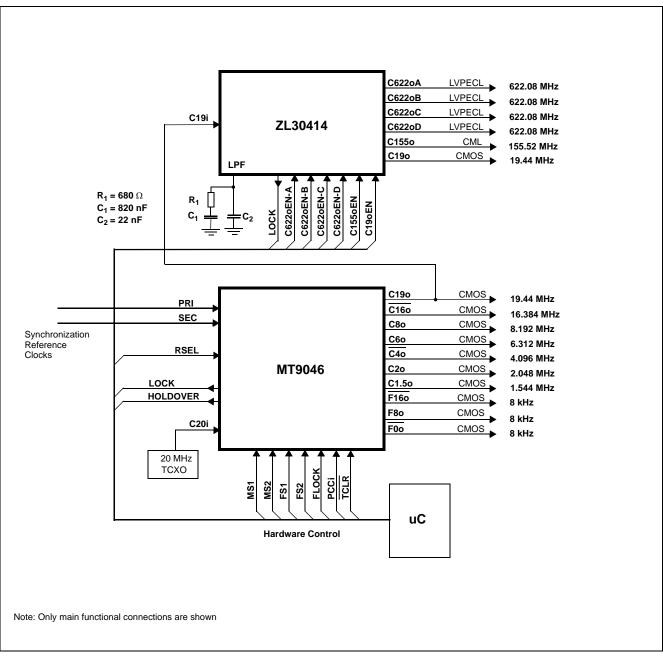
The ZL30414 in combination with the MT9046 provides an optimum solution for SONET/SDH line cards (see Figure 7).
