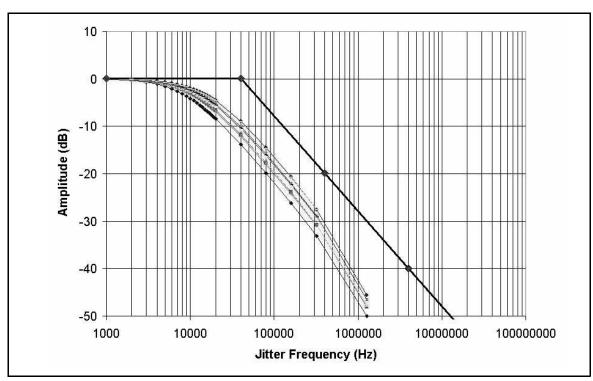
Figure 5 - Jitter Transfer Characteristic
