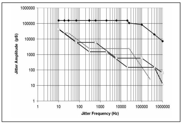
Figure 4 - Input Jitter Tolerance
