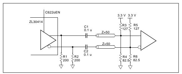
Figure 12 - Tristatable LVPECL Outputs
