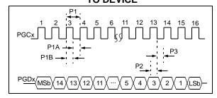
Since a 2-wire SPI is used, and data transmissions are half duplex, a simple protocol is used to control the direction of PGDx. When the programmer completes a command transmission, it releases the PGDx line and allows the programming executive to drive this line high. The programming executive keeps the PGDx line high to indicate that it is processing the command.
