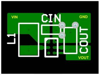
Figure 52. WLCSP Suggested Layout (Top View)
