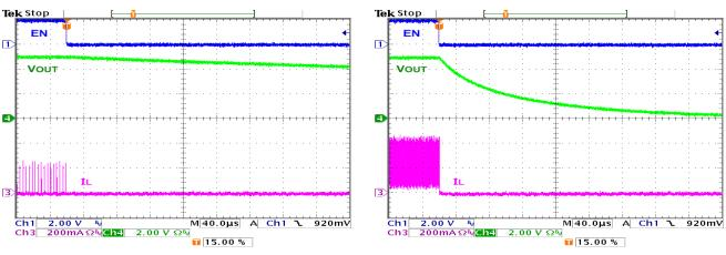
Figure 32. Shutdown, 1  $k\Omega$  Load
