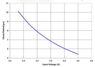
Figure 48. Fault Clock Period vs. VIN
