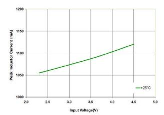
Figure 22. Maximum DC Load Current
