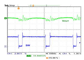
Figure 42. Output Ripple, 10 mA PFM Load
