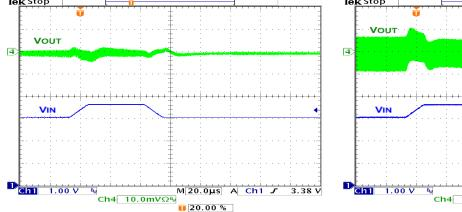
Figure 28. Line Transient, 5 mA Load, 10 µs Step
