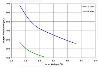
Figure 46. Output Resistance (ROUT)
