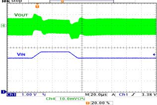
Figure 29. Line Transient, 200 mA Load, 10 µs Step
