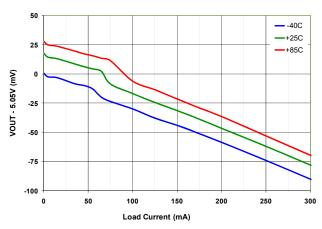
Figure 18. Line and Load Regulation
