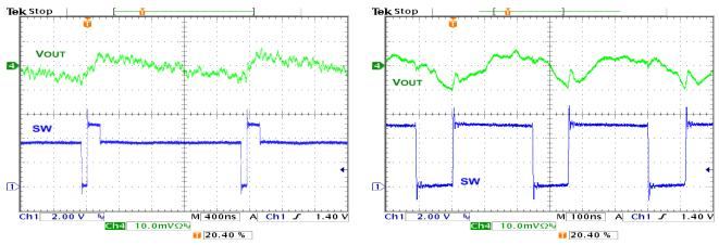
Figure 24. Output Ripple, 10 mA PFM Load
