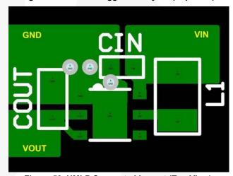
Figure 53. UMLP Suggested Layout (Top View)
