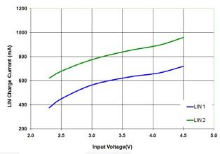
Figure 49. LIN Mode Current vs. VIN
