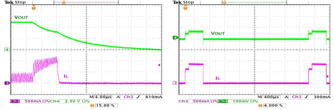
Figure 34. Overload Protection
