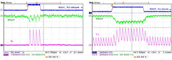
Figure 26. 0-50 mA Load Transient, 100 ns Step
