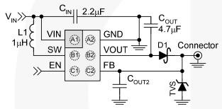
Figure 51. FAN4860 with External Transient Protection
