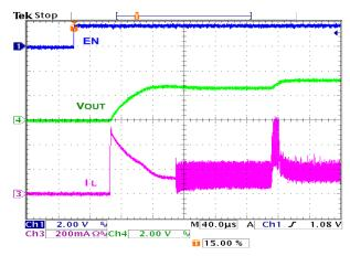
Figure 44. Startup, No Load
