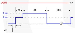
Figure 47. Fault Response into Short Circuit
