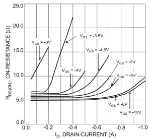
Fig. 6 On-Resistance vs. Drain-Current
